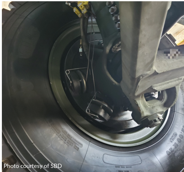
Because SBD's sphere brake is smaller, the wheel end weight is lighter. Using sphere brakes on the Stryker allows the vehicle to carry an increased payload or gain fuel efficiency, depending on the mission.
